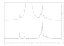
Advanced pulse sequences like the selective 1D TOCSY can be used in place of some 2D experiments, simplifying spectral analysis and allowing you to obtain your results more quickly. Shaped pulses combined with the improved linewidth of the **X-Pulse** make removing solvent peaks more effective than ever.
