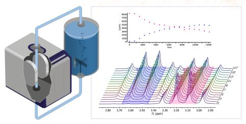
Observe your reaction at temperatures from 20°C to 70°C and with the variable temperature probe.
